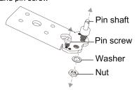
8. Insert the pin screw into the right hole and insert the pin shaft into the left hole on the lower hinge,, then secure the shaft with the washer and nut.
